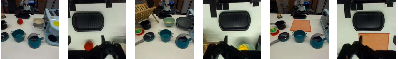
Fig. E.5: Raw observations from two different cameras for three tasks. Three (No.1, 3, 5 from the left) are from the side-view Zed2 camera and the others (No.2, 4, 6) are from Zed mini on the wrist.
