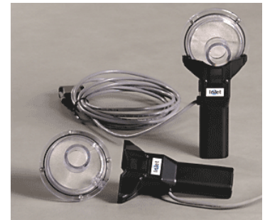
SS11LA needs 5-10 minutes to warm up; during this time, the baseline offset changes slightly.
