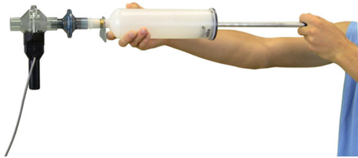
Proper handling of the Calibration Syringe Assembly
