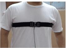
The SS5LB transducer is used to record respiration via chest or abdomen expansion and contraction. This transducer is useful for determining how deeply someone is breathing and for calculating the person's breathing rate or respiration rate. The transducer is a strain assembly that measures the change in thoracic or abdominal circumference. The strap presents minimal resistance to movement and is extremely unobtrusive.
