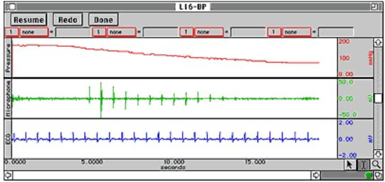
A typical blood pressure recording made using the SS19L Blood Pressure Cuff and the SS30L Electronic Stethoscope. The top channel is the cuff pressure, the middle channel is the Korotkoff sounds recording and the bottom channel shows the subject's ECG.
