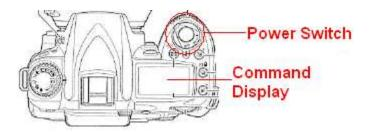
Make sure that the device is in 'Standard' mode – there should be an 'S' in the top right corner of the command display. Refer to the section on 'multiple image capture' if you are unsure.
