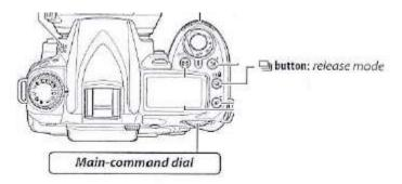
O Press and hold the 'release' button while turning the Main-command dial to switch to 'L' or 'H' mode.
