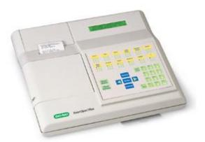
The UV/visible SmartSpec Plus spectrophotomer has a working wavelength range of 200–800 nm. It is the perfect tool for routine applications such as:
