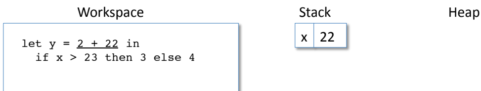
Figure 15.6: The example from Figure 15.5 after several steps of simplification. There is a binding of x to 22 in the stack, and the expression 2 + 22 is ready to simplify next.
