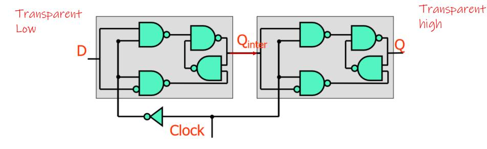
When the clock is LOW, Q<sub>inter</sub> is set to D When the clock is High, Q is set to Q<sub>inter</sub>
