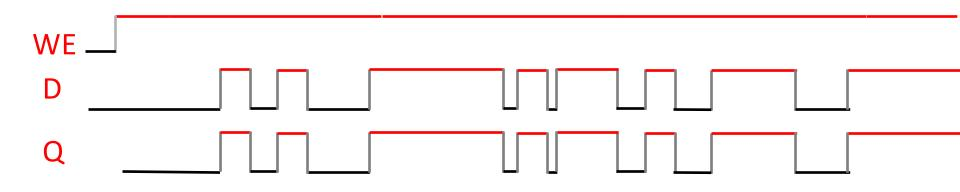
If WE were to be held at a high signal indefinitely, this would be a Fully Transparent D-Latch.
