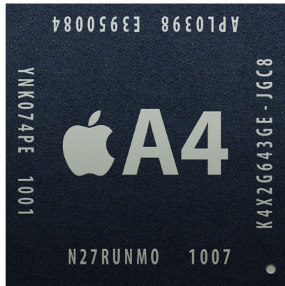
Apple A4, Armv7, 2010 Apple “Designed”, Made by Samsung
