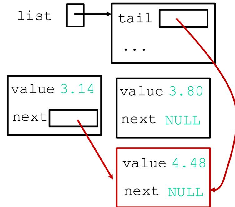
Signal handler interrupts and runs list\_push to completion...
