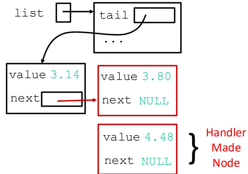
Signal handler interrupts and runs list\_push to completion...
