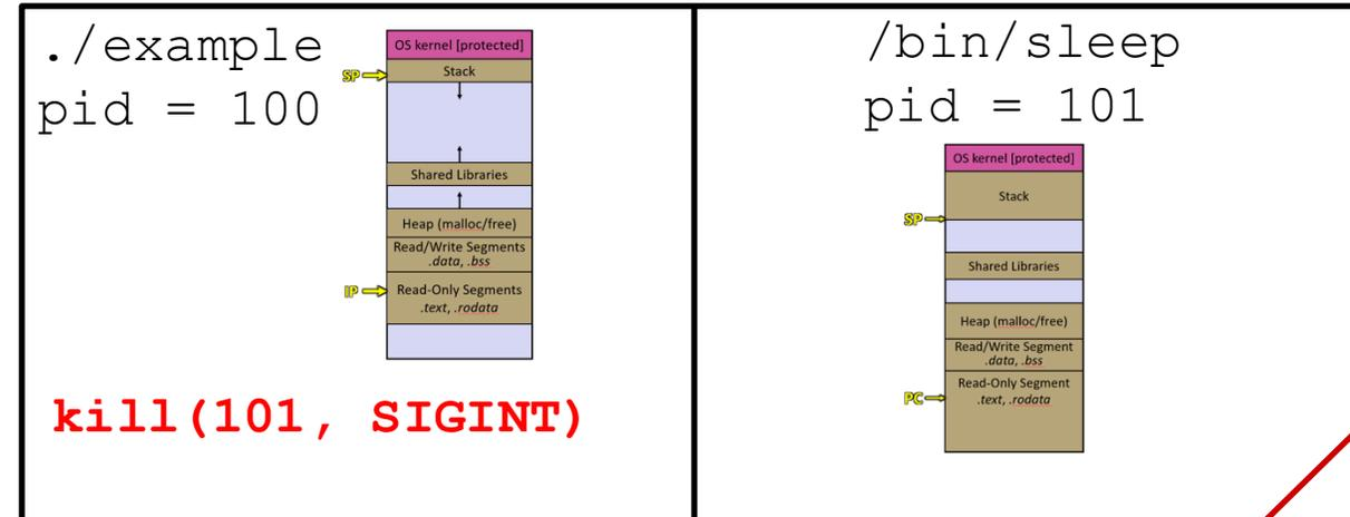
❖ './example' is attempting to send a signal to process with pid 101...
