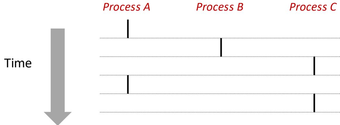
Black line indicates that the process is running during that time
