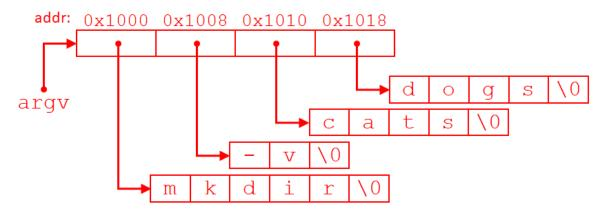
argv is the second parameter, so its value is stored in %rsi and does not take up space in memory. The character arrays have unknown/unspecified addresses that are stored in the entries of argv. Each character of the command-line arguments takes up 1 byte of memory and the elements of each character array have consecutive addresses, though the arrays are likely not contiguous to each other.
