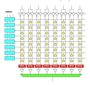
1. What is capacitance of the bit line? In terms of access transistor width  $W_{access}$ , number of words on bit line, d,  $\gamma$ , and  $C_0$ .
