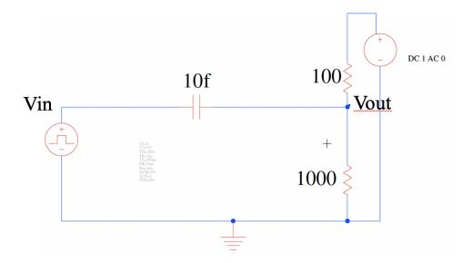
**Hints:** What is the initial voltage? What is the steady-state voltage as  $t \to \infty$ ?
