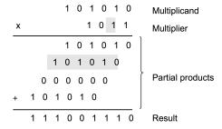
To implement the multiplication, you will design an array multiplier that multiplies two 4-bit inputs and calculates an 8-bit output. The array is shown below:
