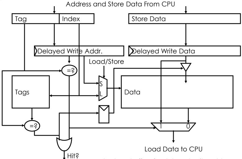
Introduce buffers for delayed write address, data. Write cache for j-th store during tag check for (j+1)-th store. Note that loads must check buffers for latest data.
